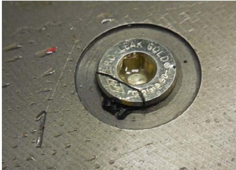
Figure 3 – Failure Mode: Typical ZLGP Extrusion
