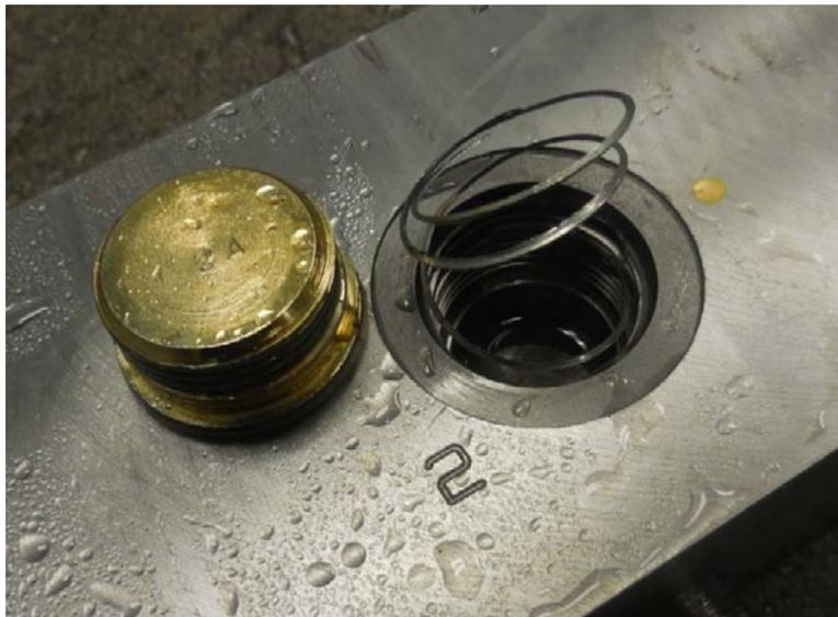
Figure 4 – Failure Mode: Typical ZLGP Ejection
