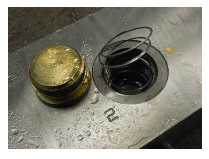
Figure 4 - Failure Mode: Typical ZLGP Ejection
