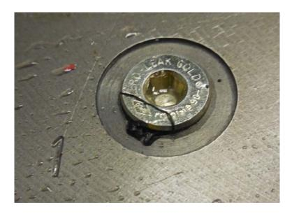
Figure 3 – Failure Mode: Typical ZLGP Extrusion
