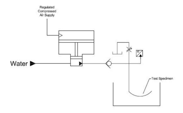
Figure 1 – Burst Test Circuit
